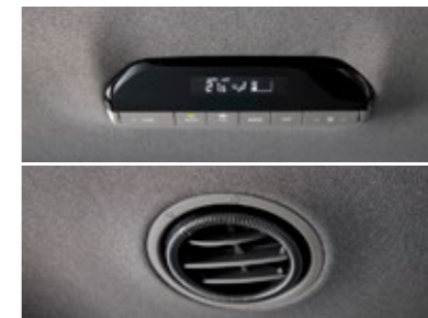
Rear Ventilation System
